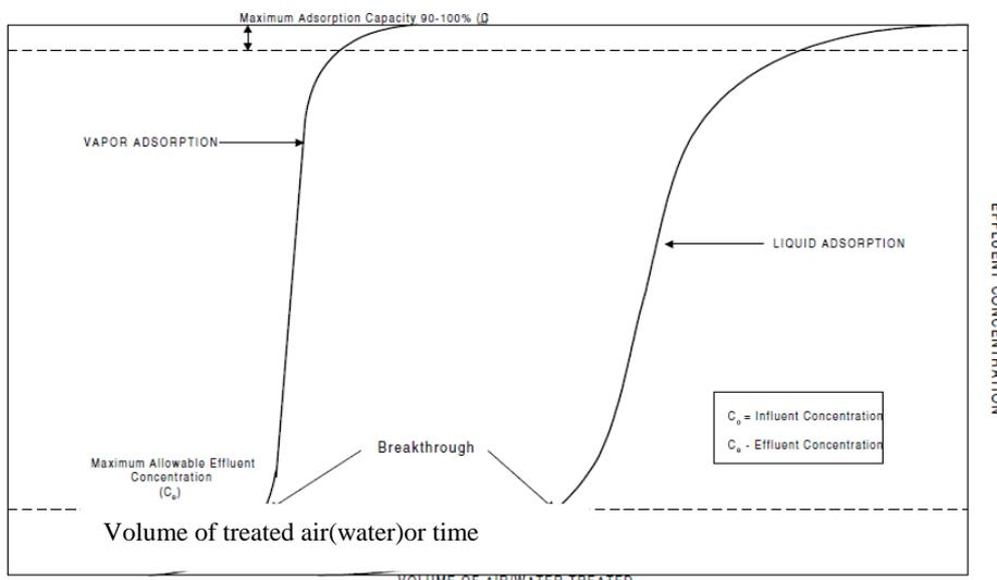
Fig (5) The Idealized Breakthrough Curve[27]
