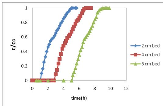
Fig (4) Breakthrough Curves Using Different Bed Heights at Temperature 25°C at Continuous Flow of 1.5l/min and 6Bar.
